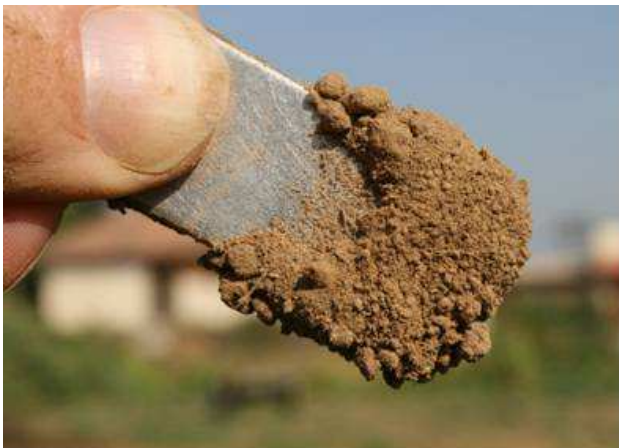
Fig.5. A paramagnetic soil sample from Maheshwar farm was almost totally drawn to a neodymium magnet.
